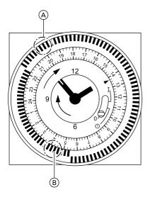
For periods when central heating is required, pull the tabs out.
