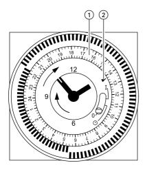
Turn ring (1) on the time switch until arrow (2) points to the current time and the hands of the clock show the current time.
