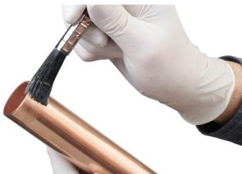
**2.** Insert the tube into the fitting until it reaches the tube stop, using a twisting action to ensure the spread of flux. Ensure the tubes are correctly lined up and adequately supported – otherwise distortion or cracking may occur when at brazing temperature.
